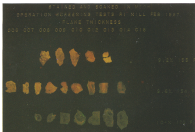
FIG. 6. Stained and soaked soybean flakes: effect of moisture content and flake thickness.
